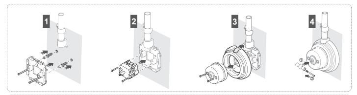
Accessories for installation with visible metallic tube Ø 16, 20 or 25 mm:
